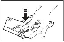
4. Line up front of cover and base. Rest cover on front edge of base as shown.
